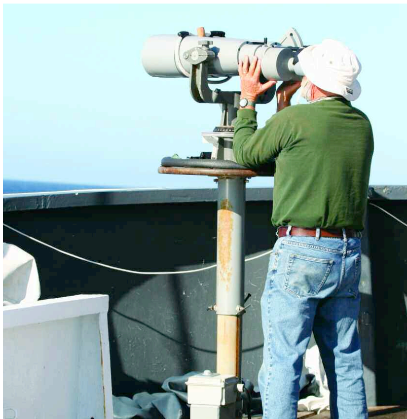
Figure 6. Gary Friedrichsen with 25 x 150 mounted binoculars used by marine mammal and seabird surveyors aboard NOAA vessels. Aply referred to as “big eyes,” these binoculars seem to result in 2–3 times the power and illumination of a single 25x telescope, allowing the identification of mammals up to 9 km (5 nmi) away and birds up to 3.7 km (2 nmi) away. Photograph by Peter Pyle © PRD, SWFSC.
