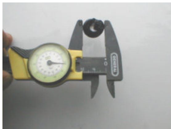
Figure 3-19. Dial caliper used to measure black turban snail shell sizes.
