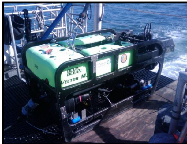
Figure 2. The Vector LV4 ROV Beagle (a) and towed camera sled (b), both of which are equipped with video cameras, lights, sizing lasers, and navigation equipment for collecting videographic imagery of the seafloor and associated organisms.
