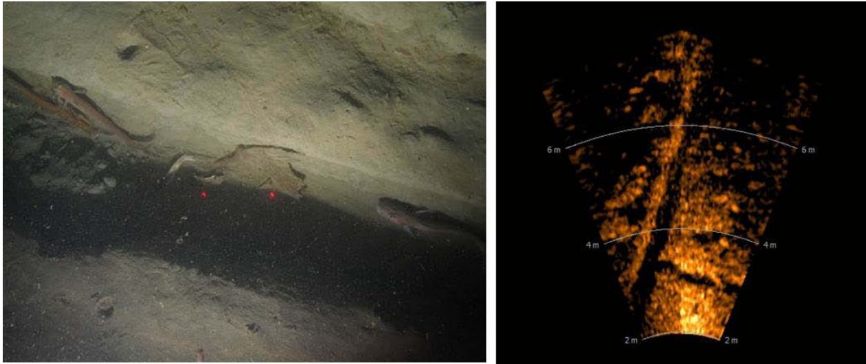
Figure 4. Trawl door scour in one of the trawled plots as depicted in an ROV still photograph (left) and ROV sonar (right).
