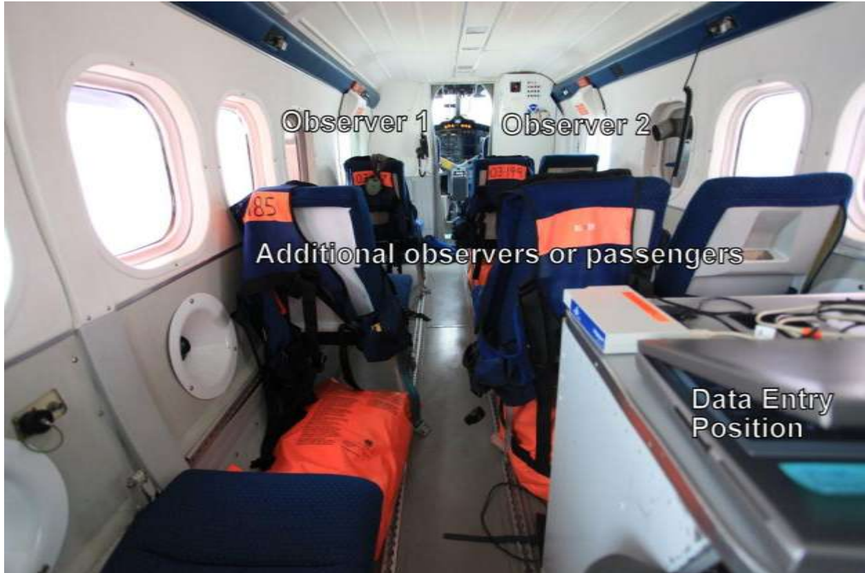
Figure 5. View of the Twin Otter's main cabin, looking forward. Observers 1 and 2 sit near the front of the cabin and view marine mammals through “bubble” windows. A data entry person sits near the rear of the plane and enters observations into a laptop. A third observer (position not seen here) lays down in the rear of the plane to view marine mammals through a plexiglass port in the belly of the plane.
