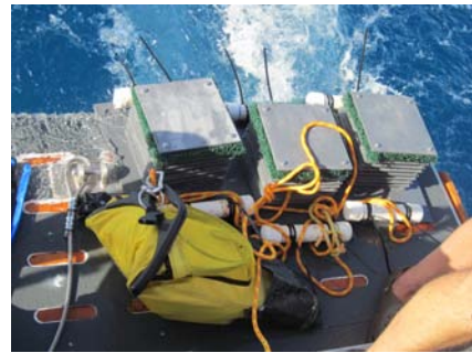
Figure 3: ARMS equipment ready for lowering off of the small boat
