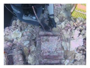
3. Remove the zip ties attaching the baseplate to the stakes.
