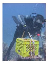
8. Attach a buoyed line to the ARMS unit for surface recover. \*\*Note: experienced divers could carry an ARMS unit to the surface during their accent and not attach a buoyed line.
