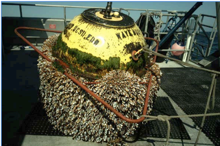
The Fulmar recovered this CDIP wave buoy off Point Sur for maintenance. Algae and barnacle colonized the buoy. Photo credit: CDIP.
