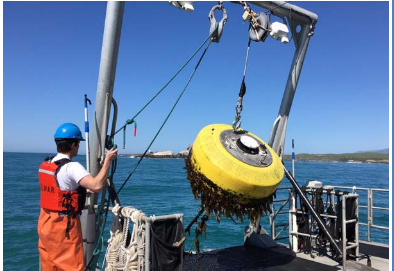
The Fulmar recovers an acoustic mooring as part of a project that tracks white sharks in national marine sanctuaries. Photo credit: ONMS.
