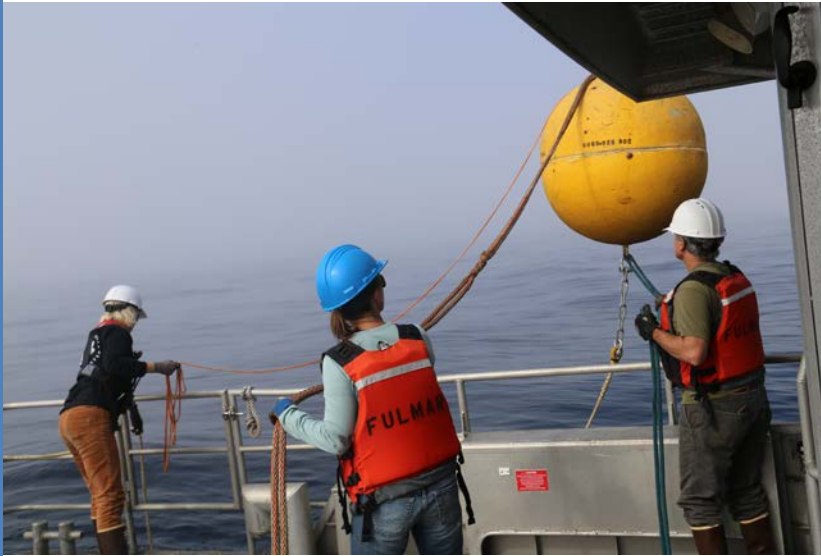
Cordell Bank NMS and PMEL researchers redeploy an acoustic mooring from the Fulmar after refurbishing its sensor on Cordell Bank.
