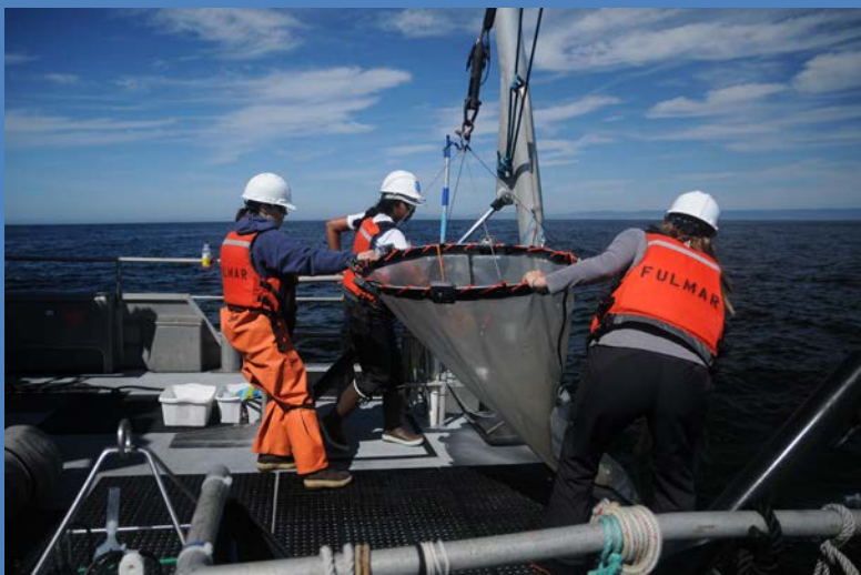
ACCESS scientists work together to recover a hoop net on the back deck of Fulmar using the A-frame and winch.
