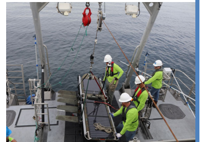
Getting ready to launch a Wave Glider using the Fulmar A Frame.
