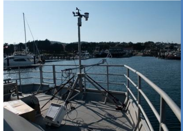
NPS installed sensors on the Fulmar's bow to monitor atmospheric turbulence. Photo credit: NPS
