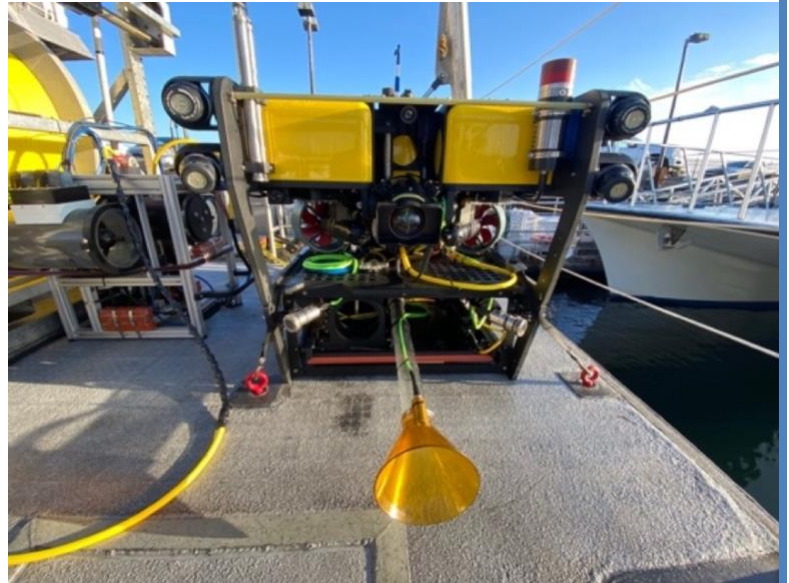
The miniROV setup on the deck of the Fulmar Photo credit: MBA/MBARI
