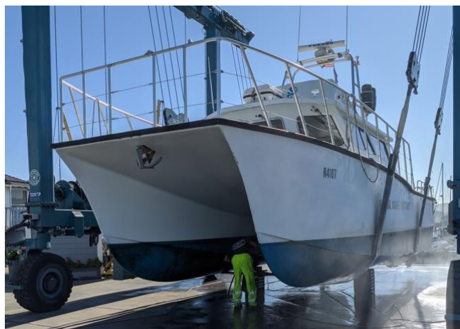
NOAA R/V R4107 hauled out at Monterey Boatyard for a hull inspection and cleaning. Photo Credit: B.Kaiser, WCRO
