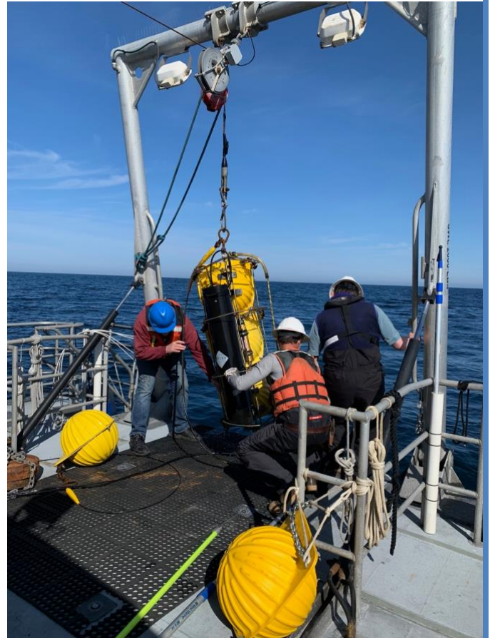
Naval Postgraduate Schools scientists recovering a HARP mooring at Sur Ridge. Photo credit: WCRO
