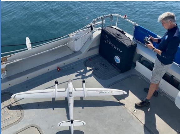
Retired NOAA Corps Officer Brian Taggart running system check for a fixed-wing UAS on the on back deck of the R4107 .
